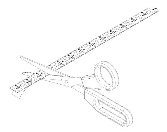
The LED strip can be separated or shortened every 20 mm. On the back of the LED strip is a double-sided heat-conducting adhesive tape, which allows installation of the LED strip. Professional LED strips can be cut with scissors.
