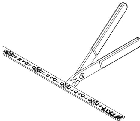
The LED strip can be separated or shortened every 45.45 mm. The connectors work on the separated parts also.
