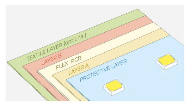
The combination of heat and pressure in our process ensures a flawless bond, encapsulating the components thoroughly while preventing any air entrapment. As a result, LumProtect® LED strips stand out in robustness and adaptability, surpassing our competitors.
