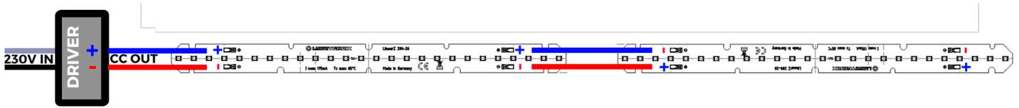
Several Lumibar strips can be connected in series to a constant current (CC) driver.
